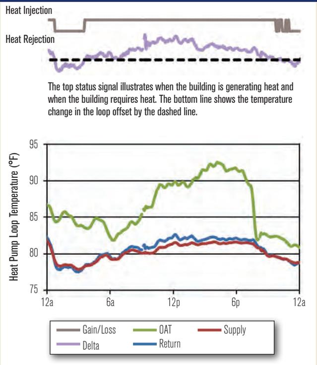
should be injecting or rejecting heat. The second signal from the top shows the temperature change in the loop offset by the dashed line. Above the dashed line, the loop is gaining heat, and below the line, the loop is losing heat. The chart shows a brown status signal on top
