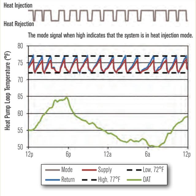
FIGURE 3 Temperature of the heat pump loop, showing the system rejecting heat when it should have been injecting heat.
