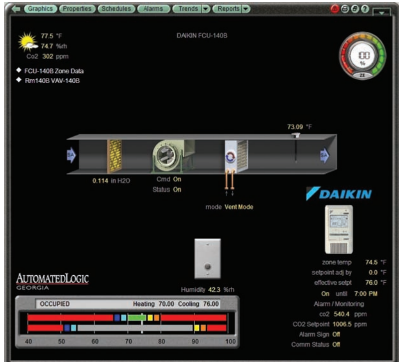
Figure 2: BACnet allows data from three vendors to be integrated in one place.
