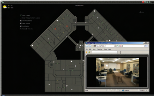
Figure 2 (left): Fire and security floor plan with CCTV image. Photo 2 (right): Facility managers have more than enough computer screens to monitor already. They don't need separate screens for every building subsystem.
