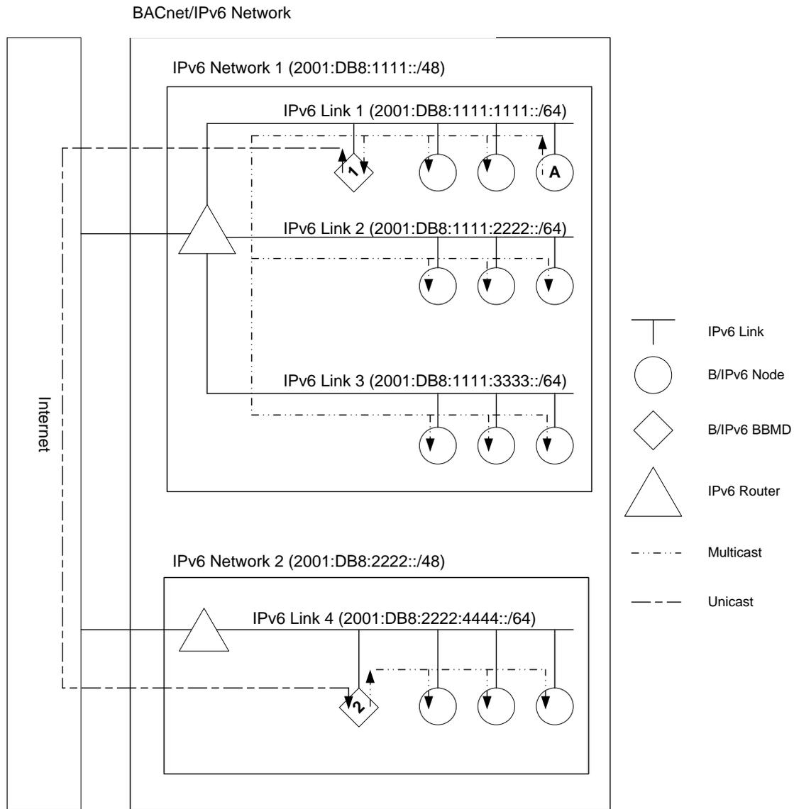
**Figure U-3.** Broadcast distribution using B/IPv6 BBMDs
