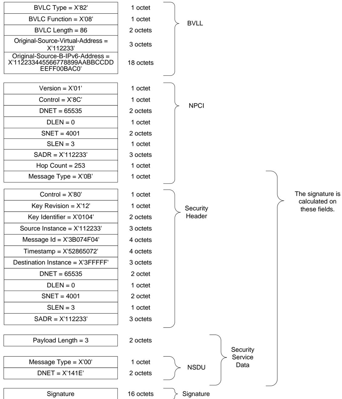
**Figure 24-Y.** An example B/IPv6 BVLL containing a Secured NPDU (Who-Is-Router-To-Network).
