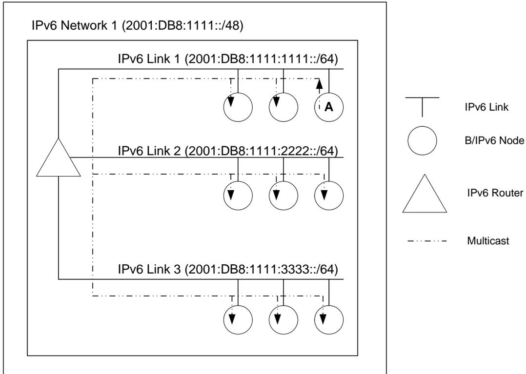
**Figure U-2.** Use of organization scope multicasts on multiple IPv6 links
