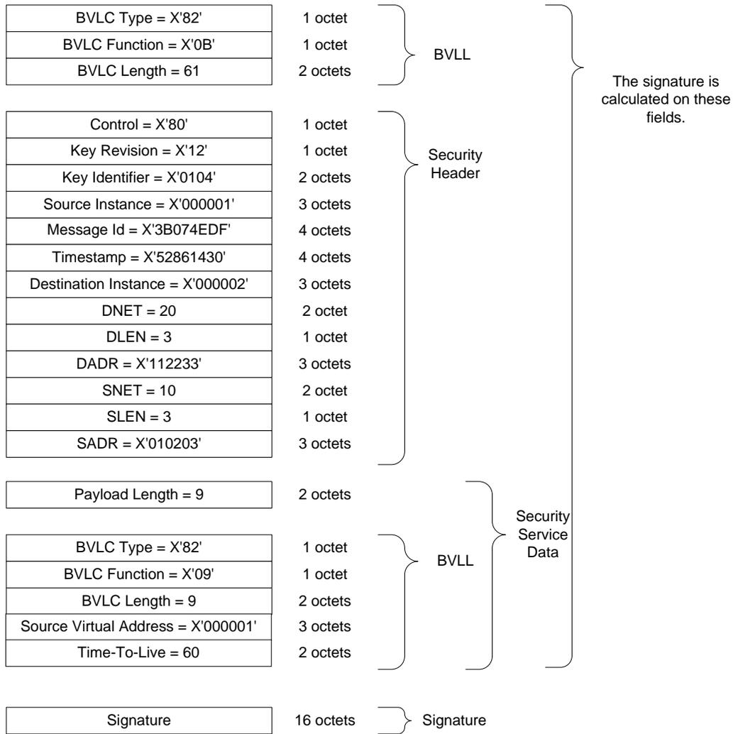
**Figure 24-X.** An example secured B/IPv6 BVLL (Register-Foreign-Device)
