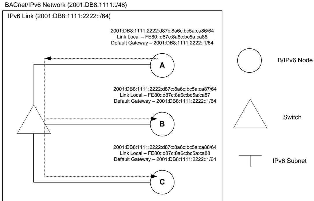
Figure U-1. Use of link-local multicasts on a single IPv6 link
